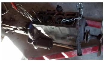
11/21/2015 – Saturday and Jim was here to continue on his engine while I worked on finishing the cleaning on Tinkerbell. Jim was successful in separating the engine from the transmission and getting the engine on the stand.
