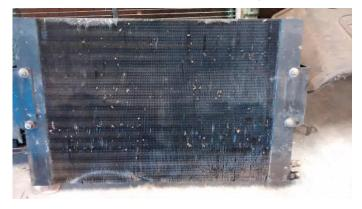
The air conditioning system did not have any standout issues to be resolved but the radiator was about like Swiss cheese. It was really bad. The new aluminum unit is due here tomorrow from the Wedge Shop and it was sorely needed. The picture tells the story.
