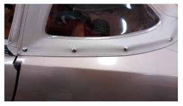
The material for the top is easily stretched when warm but it was not warm. With much trepidation the heat gun was put into use and the
