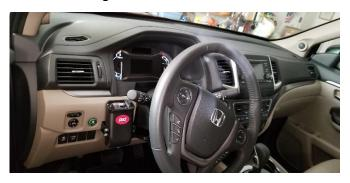
I selected a different location that still required two small holes for the mounting bracket but no other holes were needed for the harness. It is easy to reach, does not interfere with getting in or out of the truck and meets phone distance requirements. Visually it is not easily seen from passengers so it does not detract from the original look of the interior.
