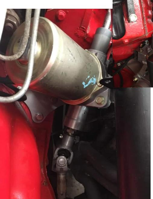
The design, and all the engineering was thanks to Dale Reardon of West coast racing, who did all the machining and just left me to do the electrics. It has transformed the way the car drives, it now feels nimble and responsive. The amount of power assistance is adjustable with a control knob under the dash.
