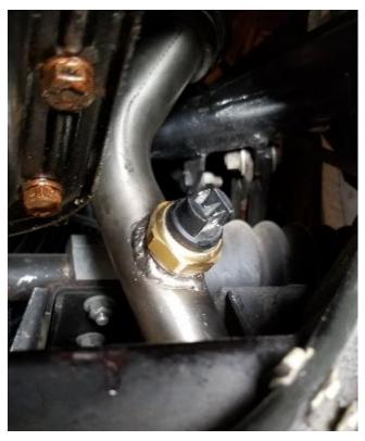
The new drain was too long to fit between the new pipe and the radiator so I cut off some of the stainless tube. Unfortunately, my tubing cutter was not big enough to use so it was hacksaw time. Some grinding was needed to clean up the slanted cut.
