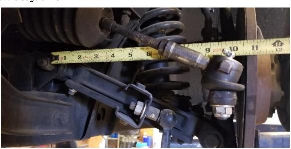
The measurement was 10 9/16ths inches. The old tie rod end was removed and the new one installed. The adjustment was to get the same distance from the disk to the hard point nut. The new part definitely travelled further onto the inner tie rod assembly than the old part to achieve the desired distance. It was locked down and I moved on to the other side.
