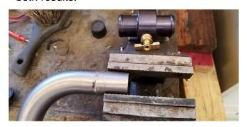
With the coolant removed the modified new system was put in place. I did modify the stainless pipe because I wanted to add a drain to the cooling system.
