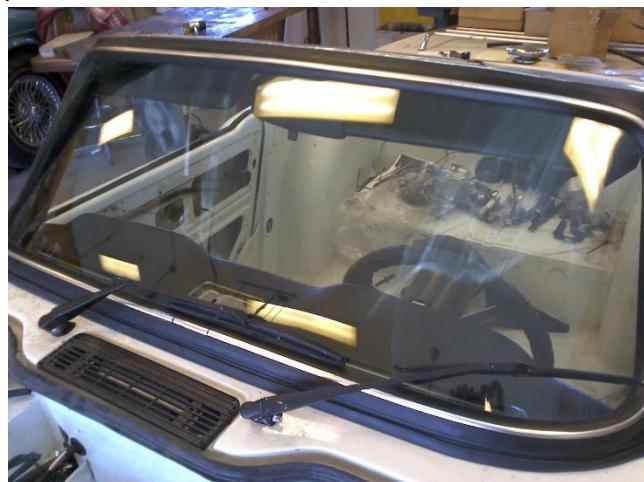
and washers were added to the main posts on either side of the assembly under the dash and all five locations tightened down. The assembly is now installed properly. The old bright strip and windshield wipers were also installed. The seal under the old windshield was also acceptable for re-use. Looks really nice Jim. Good job.
