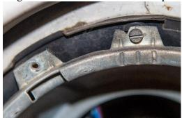
The Slotted fasteners are for headlight adjustment and should not be removed.
