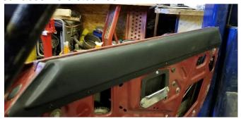
The inner and outer seals for the window glass were installed next. The process I use is to put the clips in place on the door then push the seal down into each clip. This process just seems to work better for me. It is still a pain in the butt but it is done on this door anyway.
