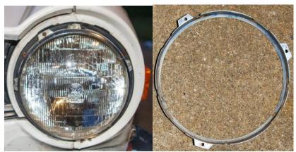
I found the headlight was retained with three Philips Head Fasteners.
