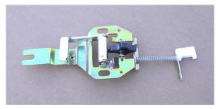
6/15/2020 – Today I thought it would be a good idea to take a look at the outside door handle to make sure it was ok before putting the door back on the car. It was not. Notice the nylon part is broken on the far left end. There is supposed to be a hole that a pin fits
