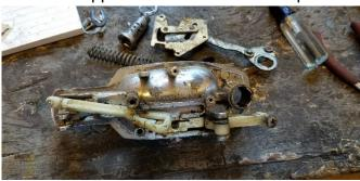
into that provides a fulcrum for the lever handle to push against the latch which releases it to open. One side of the hole is broken out.
