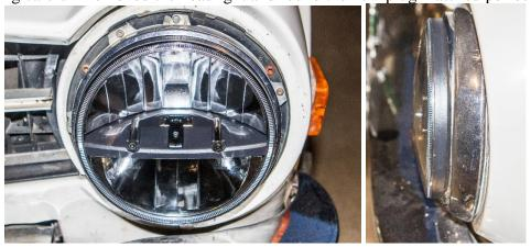
The LED headlight indexed and fit perfectly. Notice it does protrude a bit from the trim ring.
