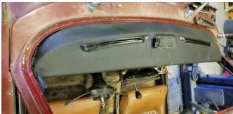
Everything is back where it is supposed to be related to the pad installation. The new windshield is on order, the door repair is in work to replace the handles on the passenger side, the left door checkstrap repair is in the "How the hell am I going to do this" stage.
