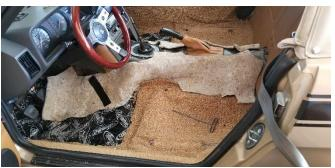
The tape on the narrow pieces is where the piece was cut to facilitate drying the carpet of coolant. I taped them back together to provide a good pattern of what I expected of the new carpet pieces.
