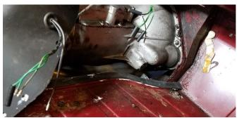
the glue holding the seal to the floor and the wiring from the transmission to the connect point hanging from the wiring harness above. The OD switch wire had not yet been routed over the heater to drop down where the green feed wire is hanging.
