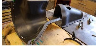
The preparation for install included gluing the seal material to the firewall edge of the bell housing cover end. As for the sides, the seal material was glued to the floor pan.
