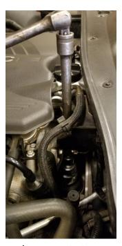
engine provides just enough access to turn the filter. The filter then lifts out and the process is reversed to install the new filter.
