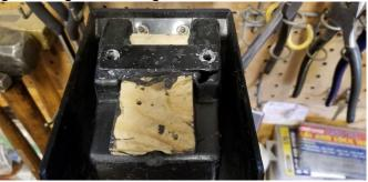
After the glue dries, holes will be drilled through the aluminum, the wood and the plastic. Countersunk bolts will hold that all together with lock nuts on the inside of the box. Or I may use ¼ inch rivets with backing plates.
