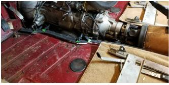
The irregular surface of the seal area made clamps a necessary support tool. I hope they do not slip over night while the
