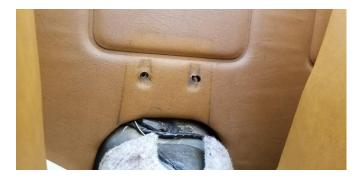
Attachment screws can then be put through the holes from the inside of the console and tightened into the bulkhead holes to finish the job.
