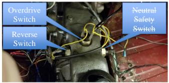
"The picture above is how the wiring was attached when the car got here. The fix was to disconnect the yellow wires on the left switch. The green reverse light wires on the right were moved to the left. That is it."
