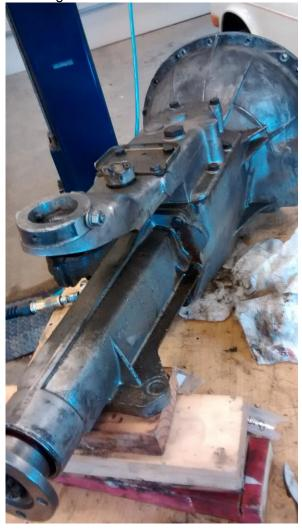
Ok, the transmission is ready to be cleaned and installed. Most of the small parts are now also cleaned and the rear engine mount is next to be removed and cleaned. Work is progressing nicely.
