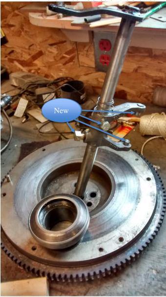
the second pin (bolt) hole could be drilled. After drilling the 5/16ths hole a bolt with a non-threaded shank was found and threaded to a precise length
