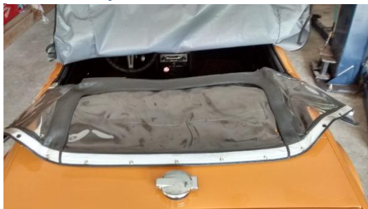
2. Fold top forward without folding back window
