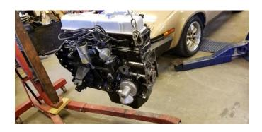
The picture above also shows a couple of issues to be resolved. The one holding up flywheel installation is a copper washer and I do not have a fuel pump yet.
