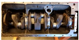
The crankshaft is fully installed as is the cam shaft, almost. The pistons, rods and rings are all assembled but not yet installed.
