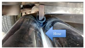
only breaking three bits in the process. After that new hose was cut and slit and holes punched on each side of the slit area to align with the hole in the flange.
