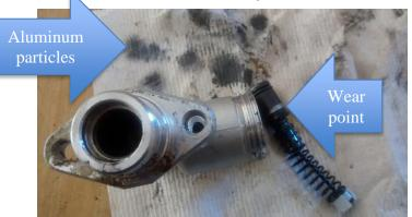
In order to clean the line and slave cylinder it had to be removed, disassembled and washed in clean brake fluid. After it was cleaned it was reassembled and reinstalled. Everything is ready for the new master cylinder which is due for deliver on Monday.
