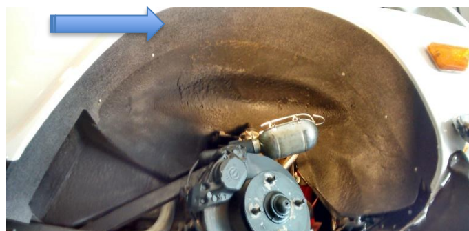
1 Aftermarket Liner Installed - Covers door sills to headlights
